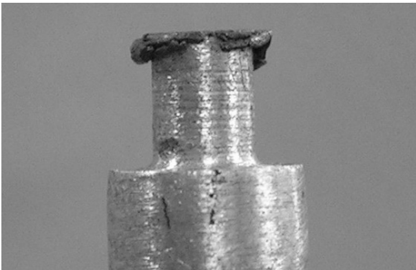
Fig. 3. Plastic deformation of pin KA356 at 1.46 MPa
